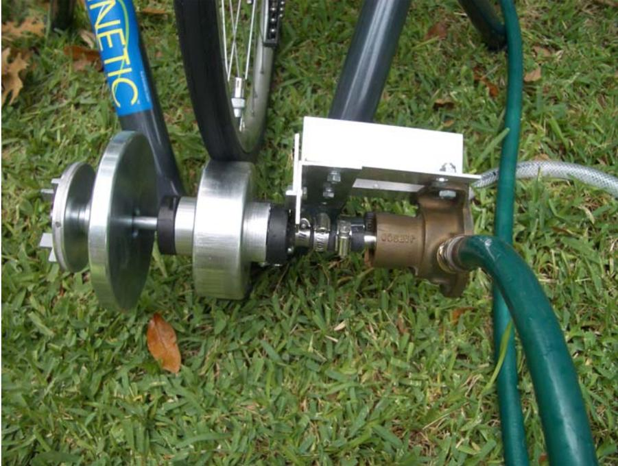
Figure 7: Pump connected to the bicycle. The plate on the left side of the roller assembly is a flywheel that helps smooth the power requirements.
