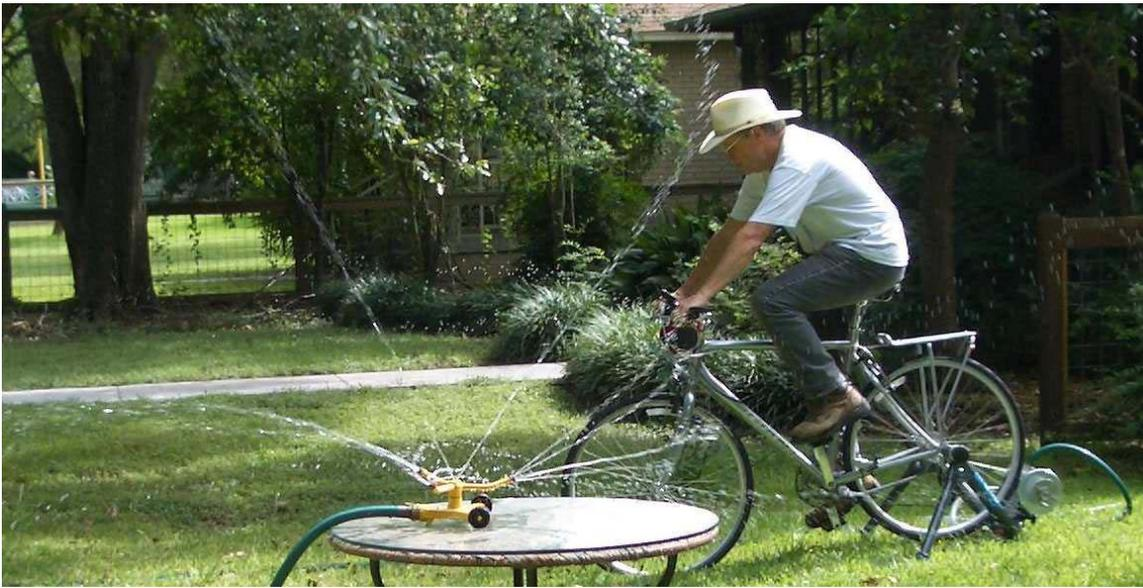
Figure 1: Shows bicycle mounted in the trainer being pedaled to operate a simple lawn sprinkler.
