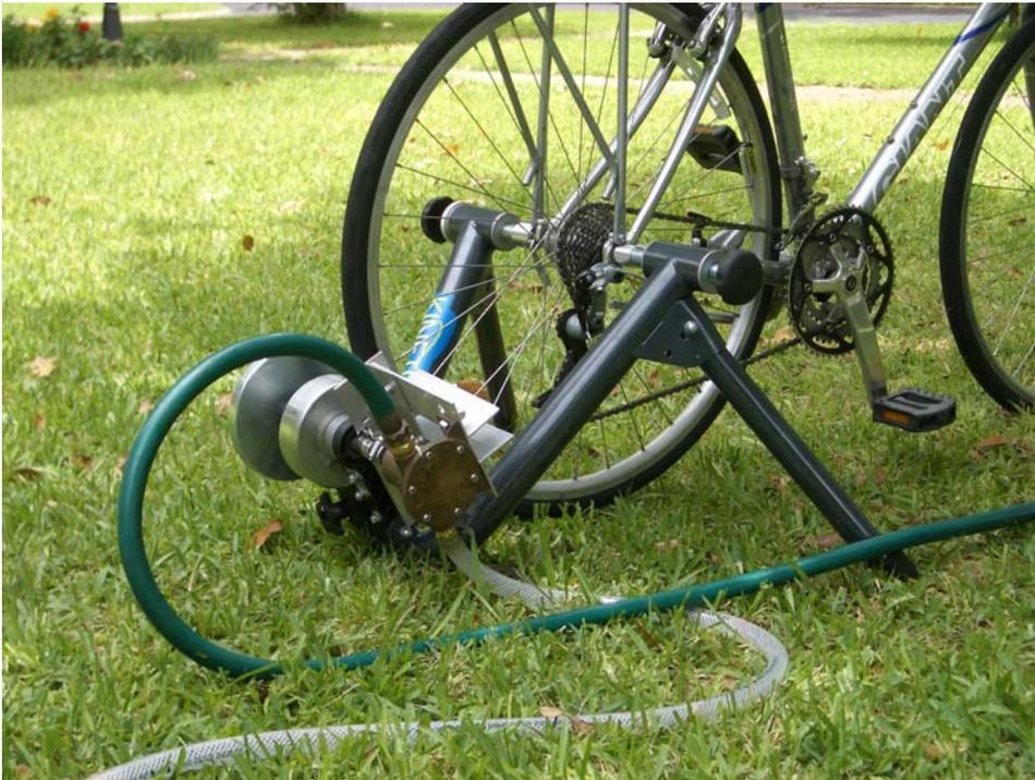
Figure 8: Ready for action. The white hose (input) is connected to a rainbarrel, the green hose to a lawn sprinkler.
