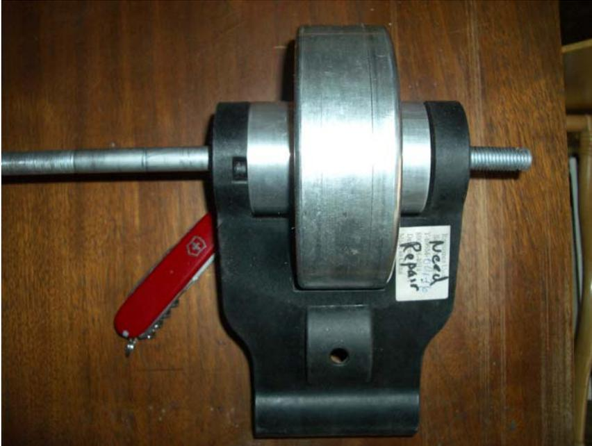
Figure 5: The roller assembly from the trainer with the fluid resistance unit and flywheel removed. The roller is approximately 4" in diameter. The roller assembly attaches to the trainer and the rear wheel of the bicycle rides on the roller, and turns it when the bicycle is pedaled.
