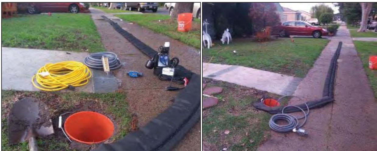
Figure 3. Equipment needed for residential stormwater runoff volume monitoring (left). Final design setup for stormwater runoff volume monitoring at a trial residential property (right).
