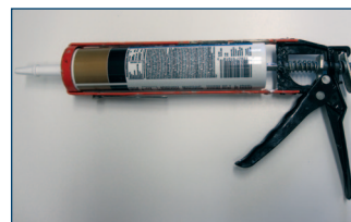
Figure 5. Caulking gun and sealant.
