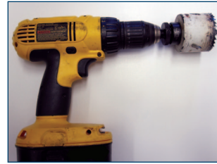
Figure 8. Drill and 2 3/8-inch hole saw.
